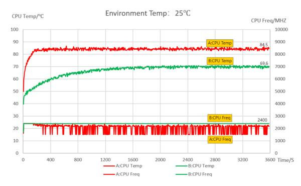
1. The following table shows the average temperature of the Raspberry Pi 5 CPU during stable operation of the two groups of devices
