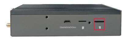
2. Press the SD card into the card slot with your hand to pop it out, and then pull out the SD card.
