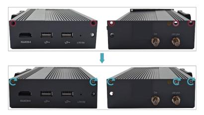
4. Align the ports on PCBA with the ports on the front panel, insert the front cover.
