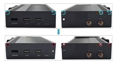
5. Remove the upper cover upward and turn it to the antenna port side.
