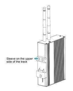
2. Press down the buckle on the lower side of the DIN-rail bracket until the bracket can be buckled on the rail, and the installation is completed.
