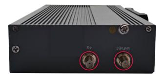
2. Align the ports on both sides of the device and the antenna and tighten them clockwise to ensure that they will not fall off.
