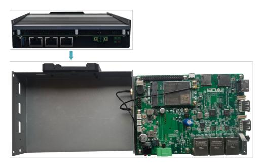
6. Use a screwdriver to loosen the 8 screws fixing the PCBA counterclockwise, remove the upper cover and flip it to the back of the PCBA.
