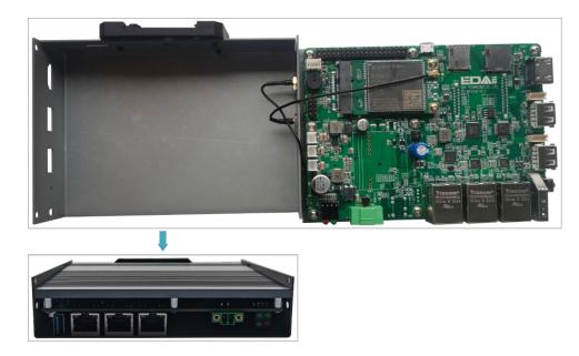
3. Align the screw holes on the upper and side panels and use a screwdriver to tighten four M2.5 screws and one grounding screw on two sides clockwise.
