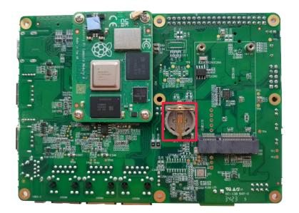
2. Put the positive pole of the battery upwards and press it into the RTC base. The installation effect is as shown below.
