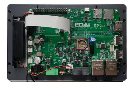
2. Put the positive pole of the battery upwards and press it into the RTC base. The installation effect is as shown below.
