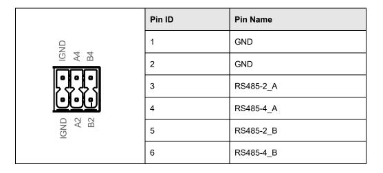
The pin names of CM4 corresponding to RS485 ports are as follows:
