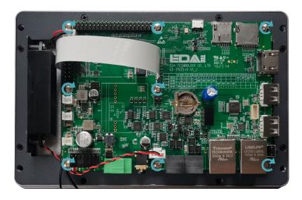
Flip the metal case upward, align the screw mounting holes on the metal case with the screw mounting holes on the back of the LCD screen, and cover it downward on the back of the LCD screen.
