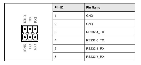
The pin names of CM4 corresponding to RS232 ports are as follows:
