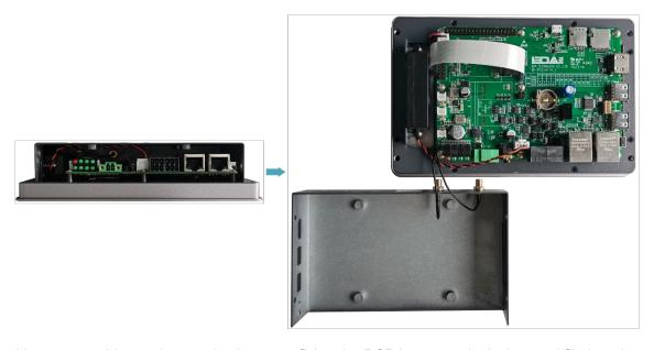
6. Use a screwdriver to loosen the 8 screws fixing the PCBA counterclockwise, and flip it to the back of the PCBA.
