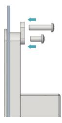
5. Use 4 M4x8 screws to pass through the buckle and tighten it clockwise to fix the buckle to the device; then use 4 M4x16 screws to pass through the screw hole (threaded hole) of the buckle and tighten clockwise to the end through the buckles.
