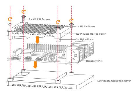
①Place the **Raspberry Pi 4** on the **ED-Pi4Case-OB Bottom Cover** by aligning it with the pre-drilled holes on the **ED-Pi4Case-OB Bottom Cover**.
