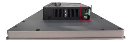
5. Use a screwdriver to tighten 2 M3 screws clockwise to fix the side cover.
