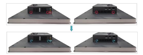
4. Align the ports on the PCBA with the port's holes on the side panel, and insert the side cover.
