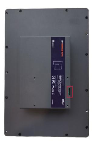
2. Insert the SD card into the corresponding card slot with the contact side facing down, making
