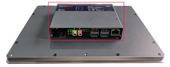
3. Use a screwdriver to tighten four M3 screws and one grounding screw on two sides clockwise.
