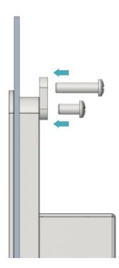
5. Use 4 M4x8 screws to pass through the buckle and tighten it clockwise to fix the buckle to the device; then use 4 M4x16 screws to pass through the screw hole (threaded hole) of the
