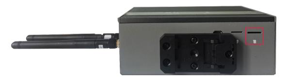
2. Insert the Micro SD card with the chip side up into the corresponding card slot, and hear a sound to indicate that the installation is complete.
