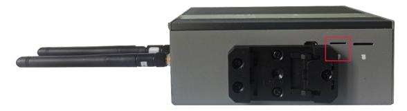
2. Insert the Nano SIM card with the chip side up into the corresponding card slot, and hear a sound to indicate that the installation is complete.
