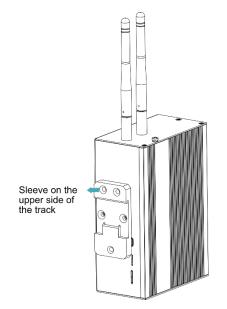
2. Press down the buckle on the lower side of the DIN-rail bracket until the bracket can be buckled on the rail, and the installation is completed.
