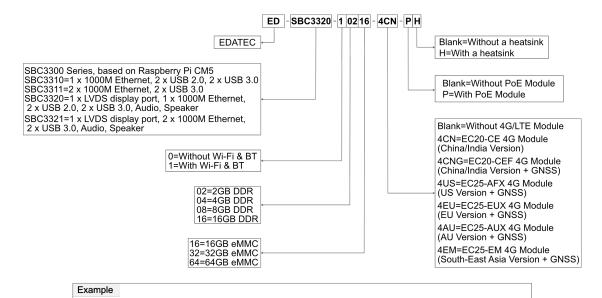
Configuration: Mini-ITX Industrial Single Board Computer Based on Raspberry Pi CM5, with Wi-Fi & Bluetooth,
