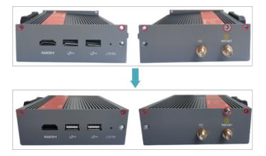
3. Align the ports on PCBA with the ports on the front panel, insert the front cover, and then use a screwdriver to fasten two M3 screws clockwise, as shown in the following figure.
