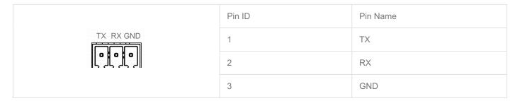
The pin names of Pi5 corresponding to RS232 interface are as follows:
