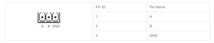
The pin names of Pi5 corresponding to RS485 interface are as follows:
