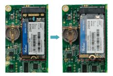
4. Insert the screws that secure the SSD and tighten clockwise to secure the SSD to the PCBA.
