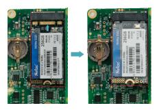
4. Insert the screws that secure the SSD and tighten clockwise to secure the SSD to the PCBA.
