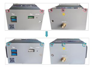
3. Align the ports on PCBA with the ports on the front panel, insert the front cover, and then use a screwdriver to fasten two M3 screws clockwise, as shown in the following figure.
