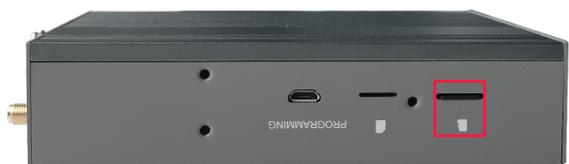
2. Press the Micro SD card into the card slot with your hand to pop it out, and then pull out the Micro SD card.
