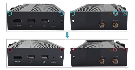
5. Remove the upper cover upward and turn it to the antenna port side.
