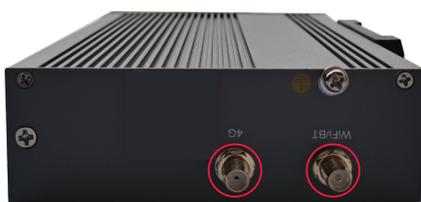
2. Align the ports on both sides of the device and the antenna and tighten them clockwise to ensure that they will not fall off.
