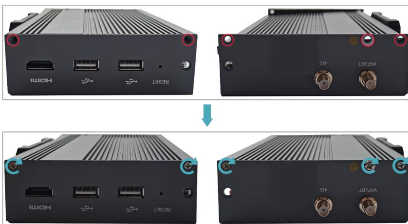
4. Align the ports on PCBA with the ports on the front panel, insert the front cover.
