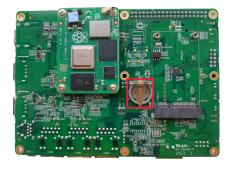
2. Put the positive pole of the battery upwards and press it into the RTC base. The installation effect is as shown below.
