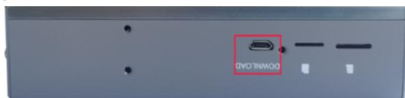
3. Connect the power cord and USB flashing cable (Micro-USB to USB Type-A).
