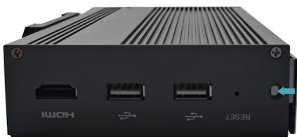
5. Insert 2 M3 screws and then use a screwdriver to fasten two M3 screws clockwise.
