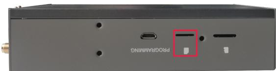
3. Insert the Nano SIM card into the corresponding card slot with the chip side up, and hear a sound to indicate that the installation is completed.
