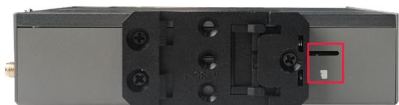
2. Insert the Micro SD card into the corresponding card slot with the contact side facing down, and hear a sound to indicate that the installation is completed.
