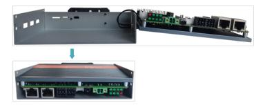
2. Align the screw holes on the upper and side panels, and use a screwdriver to tighten four M2.5 screws and one grounding screw on two sides clockwise, as shown in the following figure.
