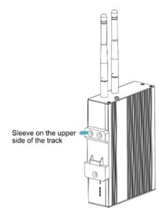
2. Press down the buckle on the lower side of the DIN-rail bracket until the bracket can be buckled on the rail, and the installation is completed.
