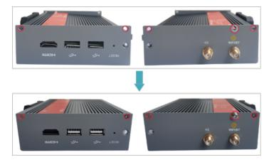
3. Align the ports on PCBA with the ports on the front panel, insert the front cover, and then use a screwdriver to fasten two M3 screws clockwise, as shown in the following figure.
