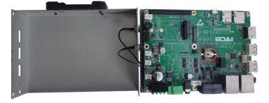
2. Put the positive pole of the battery upwards and press it into the RTC base. The installation effect is as shown below.
