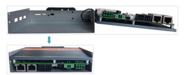
2. Align the screw holes on the upper and side panels, and use a screwdriver to tighten four M2.5 screws and one grounding screw on two sides clockwise, as shown in the following figure.
