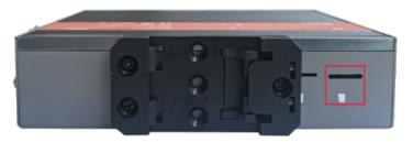
2. Insert the Micro SD card with the front face down into the corresponding card slot, and hear a sound to indicate that the installation is complete.
