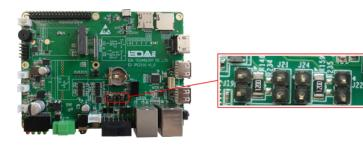
The corresponding relationship between  $120\Omega$  terminal resistance and serial port is as follows:
