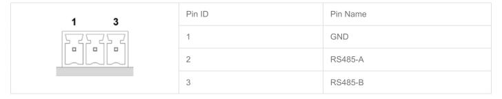
The pin names corresponding to the RS485 interface on the CM0 are as follows:
