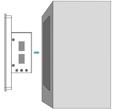
4. Align the screw hole (unthreaded hole) of the buckles with the buckle mounting holes on the device side.
