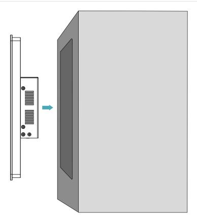
4. Align the screw holes (non-threaded) of the buckles with the buckle mounting holes on the device side.
