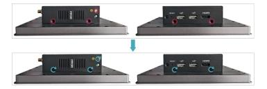
4. Align the ports on PCBA with the ports on the side panel, insert the side cover.
