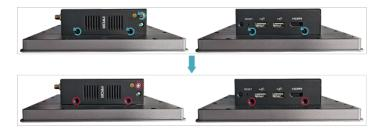
5. Remove the metal case upward and turn it to the ports side.
