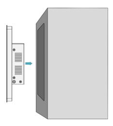
4. Align the screw hole (unthreaded hole) of the buckle with the buckle mounting hole on the side of the device.
