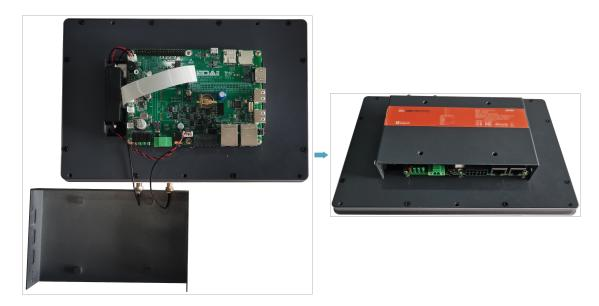
3. Align the screw holes on side panels of metal case, insert 4 M3 screws and one grounding screw, then tighten clockwise with a screwdriver.
