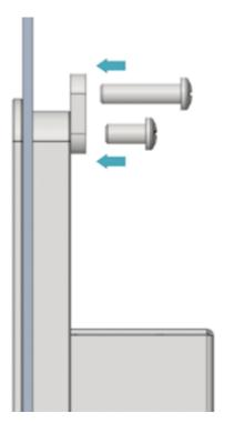
5. Use 4 M4\*10 screws to pass through the buckle and tighten it clockwise to fix the buckle to the device; then use 4 M4\*16 screws to pass through the screw hole (threaded hole) of the buckle and tighten clockwise to the end through the buckles.
