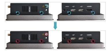
5. Remove the metal case upward and turn it to the ports side.
