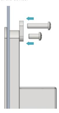
5. Use 4 M4\*10 screws to pass through the buckle and tighten it clockwise to fix the buckle to the device; then use 4 M4\*16 screws to pass through the screw hole (threaded hole) of the buckle and tighten clockwise to the end through the buckles.
