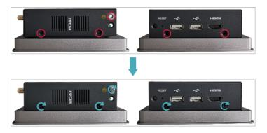
4. Align the ports on PCBA with the ports on the side panel, insert the side cover.
