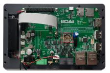
2. Put the positive pole of the battery upwards and press it into the RTC base. The installation effect is as shown below.
