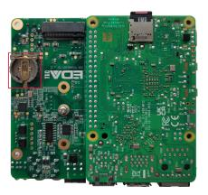
2. Place the positive terminal of the battery facing up, and press it into the RTC base. The completed installation is as shown below.
