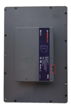
2. Insert the Micro SD card into the corresponding card slot with the contact side facing up, making sure it will not fall out.
