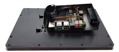
6. Use a screwdriver to loosen 6 screws of PCBA mounting counterclockwise to separate the PCBA from the metal case, and flip it to the back of PCBA.
