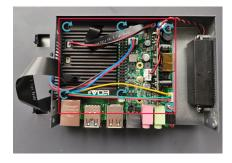
2. Flip the metal case downward, align the screw mounting holes on the metal case with the screw mounting holes on the back of the LCD screen, and cover it downward on the back of the LCD screen.
