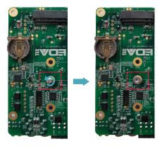
3. Insert the SSD into the connector with the contacts facing up.
