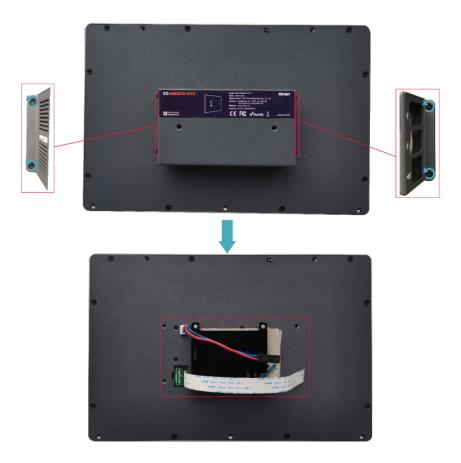
3. Use a screwdriver to loosen 4 M2.5 screws on passive cooler counterclockwise, and remove the passive cooler.
