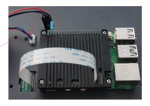
9. Cover the case, insert 4 M3 screws, and tighten clockwise to fix the case to the back of the LCD screen.
