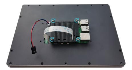
8. Plug the power cord into the corresponding 40-Pin on the Raspberry Pi 5.
