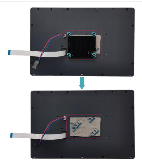
4. Remove the film of thermal conductive silicone.
