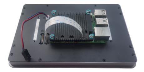
8. Plug the power cord into the corresponding 40-Pin on the Raspberry Pi 5.
