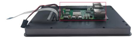
6. Pass the FPC cable through the reserved hole on the passive cooler, insert it into the CAM/ DISP1 port on the Raspberry Pi 5, and then place the passive cooler on the Raspberry Pi 5 (make sure the four mounting holes of the passive cooler are aligned with 4 mounting holes of Raspberry Pi 5).
