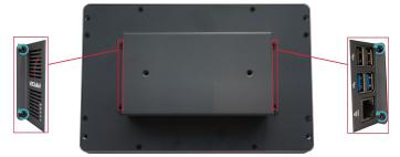
b. Locate the SD card location and remove the SD card with tweezers.
