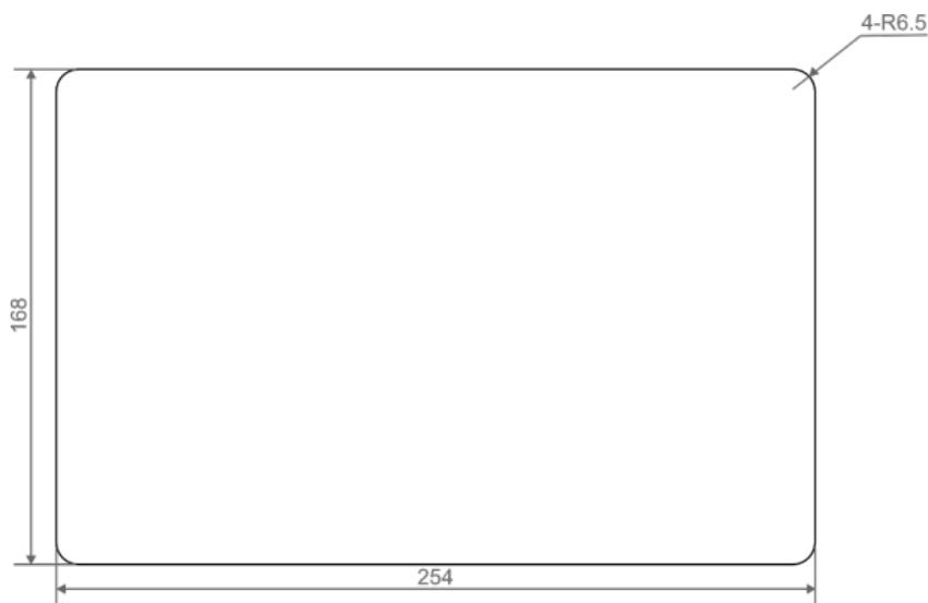
2. Drill a hole on the cabinet according to the aperture size defined in Step 1.
