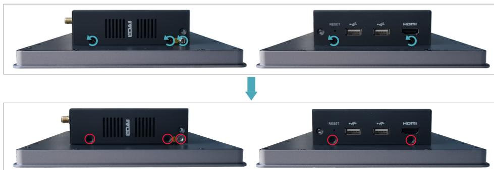
5. Remove the metal case upward and turn it to the antenna port side.
