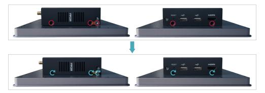
4. Align the ports on PCBA with the ports on the side panel, insert the side cover.
