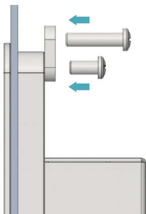
5. Insert four M4\*10 screws through the unthreaded holes of the buckle. Tighten clockwise with a screwdriver to secure the buckle to the device. Then, insert four M4\*16 screws through the threaded holes of the buckle. Press them against the inner surface of the cabinet chassis and drive clockwise with a screwdriver until full thread engagement is achieved.
