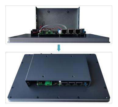
3. Align the screw holes on side panels of metal case, insert 4 M3 screws and one grounding screw, then tighten clockwise with a screwdriver.
