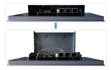
6. Use a screwdriver to loosen the 8 screws fixing the PCBA counterclockwise, and flip it to the back of the PCBA.
