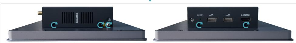
4. Align the ports on PCBA with the ports on the side panel, insert the side cover.
