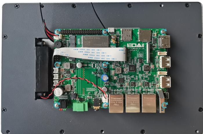
2. Flip the metal case downward, align the screw mounting holes on the metal case with the screw mounting holes on the back of the LCD screen, and cover it downward on the back of the LCD screen.
