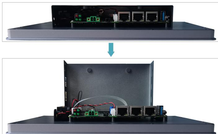
6. Use a screwdriver to loosen the 8 screws fixing the PCBA counterclockwise, and flip it to the back of the PCBA.
