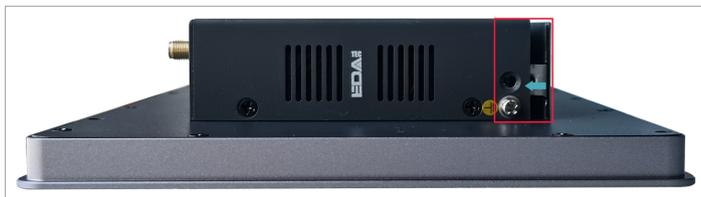
5. Insert 2 M3 screws and then use a screwdriver to tighten two M3 screws clockwise.
