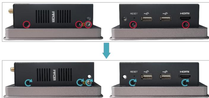
4. Align the ports on PCBA with the ports on the side panel, insert the side cover.
