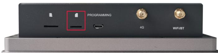
2. Insert the Nano SIM card into the corresponding card slot with the chip side up, and hear a sound to indicate that the installation is completed.
