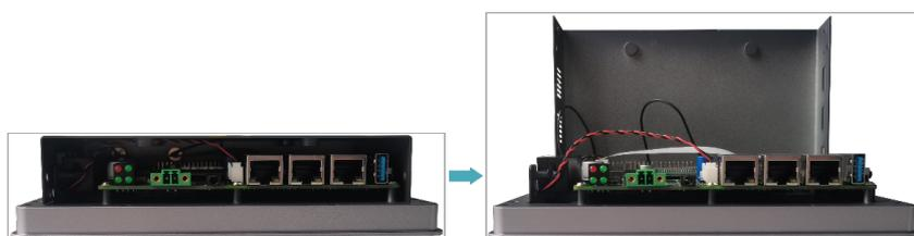
6. Use a screwdriver to loosen the 8 screws fixing the PCBA counterclockwise, and flip it to the back of the PCBA.
