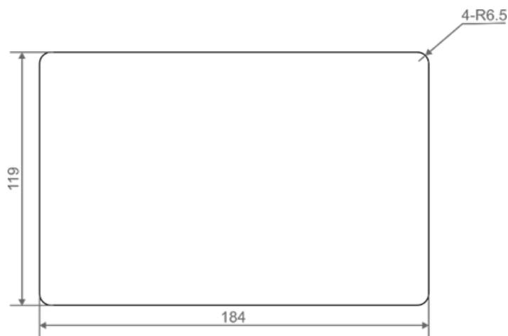
2. Drill a hole on the cabinet according to the aperture size defined in Step 1.
