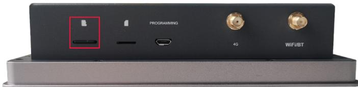
2. Press the SD card into the card slot with your hand to pop it out, and then pull out the Micro SD card.
