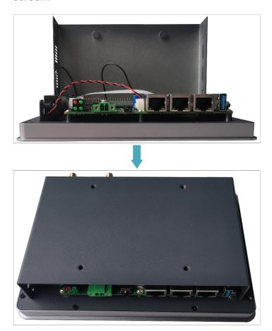
3. Align the screw holes on side panels of metal case, insert 4 M3 screws and one grounding screw, then tighten clockwise with a screwdriver.
