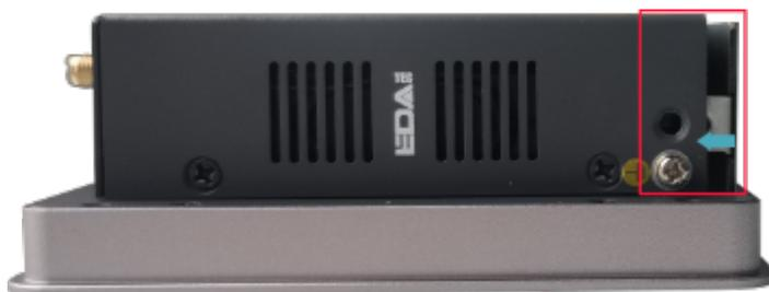
5. Insert 2 M3 screws and then use a screwdriver to tighten two M3 screws clockwise.
