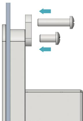
5. Insert four M4\*10 screws through the unthreaded holes of the buckle. Tighten clockwise with a screwdriver to secure the buckle to the device. Then, insert four M4\*16 screws through the threaded holes of the buckle. Press them against the inner surface of the cabinet chassis and drive clockwise with a screwdriver until full thread engagement is achieved.
