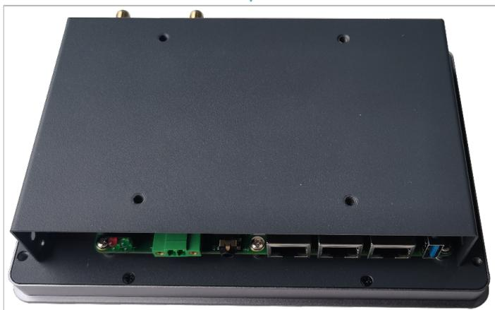
3. Align the screw holes on side panels of metal case, insert 4 M3 screws and one grounding screw, then tighten clockwise with a screwdriver.
