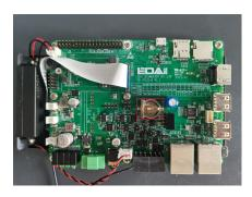
2. Put the positive pole of the battery upwards and press it into the RTC base. The installation effect is as shown below.
