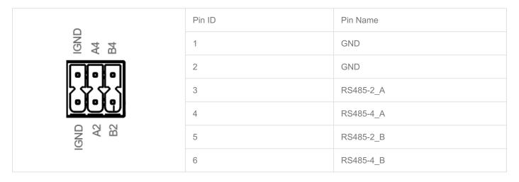
The pin names of CM4 corresponding to RS485 interface are as follows:
