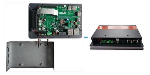
3. Align the screw holes on side panels of metal case, insert 4 M3 screws and one grounding screw, then tighten clockwise with a screwdriver.
