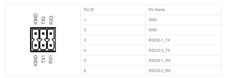
The pin names of CM4 corresponding to RS232 interface are as follows:
