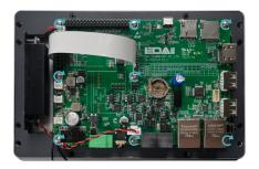
2. Flip the metal case upward, align the screw mounting holes on the metal case with the screw mounting holes on the back of the LCD screen, and cover it downward on the back of the LCD screen.
