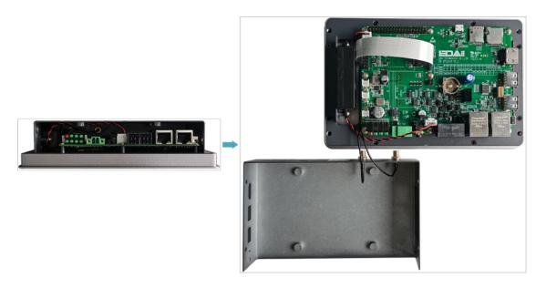
6. Use a screwdriver to loosen the 8 screws fixing the PCBA counterclockwise, and flip it to the back of the PCBA.
