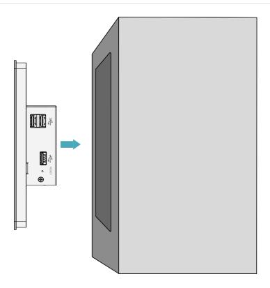
4. Align the screw holes (non-threaded) of the buckles with the buckle mounting holes on the device side.
