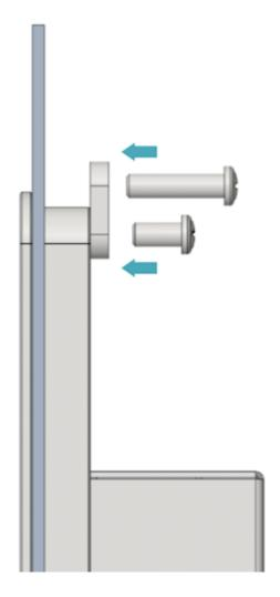
5. Use 4 M4\*10 screws to pass through the buckle and tighten it clockwise to fix the buckle to the device; then use 4 M4\*16 screws to pass through the screw hole (threaded hole) of the buckle and tighten clockwise to the end through the buckles.
