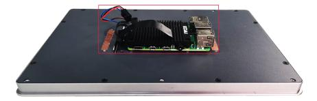
8. Insert 3 M2.5\*12 screws and 1 M2.5\*5 screw, then tighten them clockwise to secure the Raspberry Pi 4 and ED-Pi4PCOOLER to the back side of the LCD screen.
