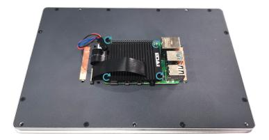
9. Plug the power cord into the corresponding 40-Pin on the Raspberry Pi 4.
