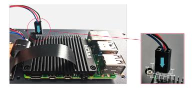
10. Cover the case, insert 4 M3 screws, and tighten clockwise to fix the case to the back of the LCD screen.
