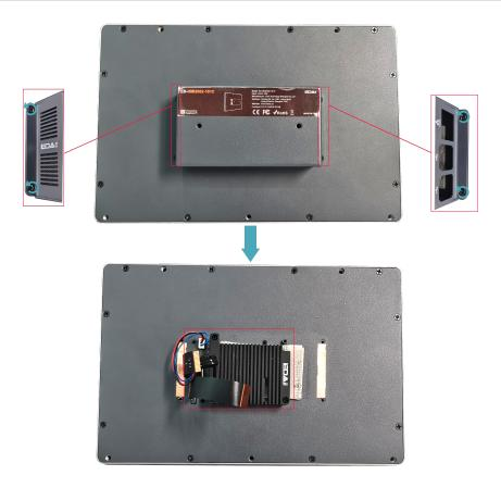
3. Use a screwdriver to loosen 3 M2.5 screws on ED-Pi4PCOOLER counterclockwise, and remove the cooler.
