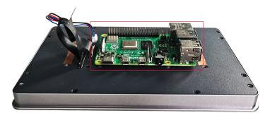
5. Pass the FPC cable through the reserved hole on the ED-Pi4PCOOLER.
