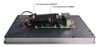
6. Plug the FPC cable into the CAMERA and DISPLAY ports of the Raspberry Pi 4 respectively.
