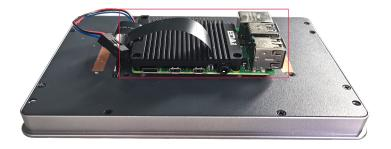
8. Insert 3 M2.5\*12 screws and 1 M2.5\*5 screw, then tighten them clockwise to secure the Raspberry Pi 4 and ED-Pi4PCOOLER to the back side of the LCD screen.
