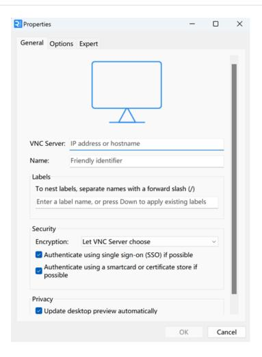
2. After entering the IP address of ED-HMI2002-070C, click "OK".
