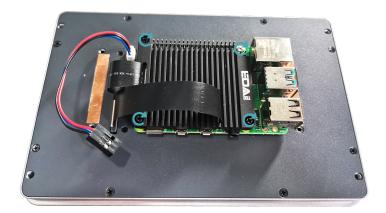
9. Plug the power cord into the corresponding 40-Pin on the Raspberry Pi 4.
