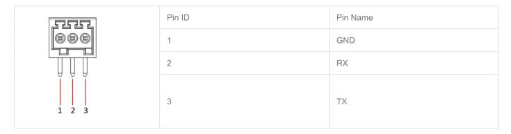
The pin names of CM4 corresponding to RS232 interface are as follows:
