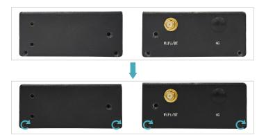
4. Make the connector on the PCBA align with the connector position on the front panel, insert the front cover. Then align the rail bracket with the screw holes on the side, insert the 4 M3 screws, and finally use a screwdriver to tighten the 4 M3 screws on the two sides clockwise, as shown in the figure below.
