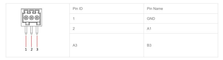
The pin names of CM4 corresponding to RS485-3 interface are as follows:
