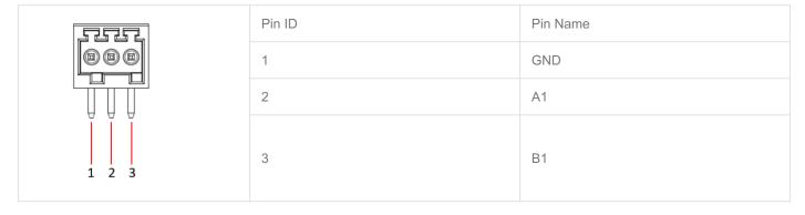
The pin names of CM4 corresponding to RS485-1 interface are as follows:
