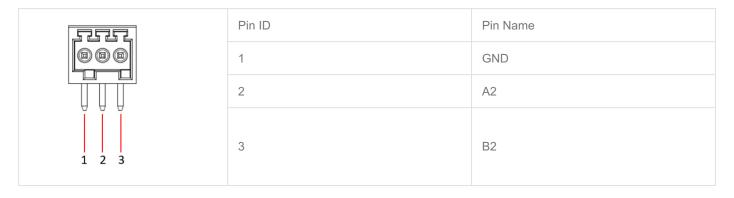
The pin names of CM4 corresponding to RS485-2 interface are as follows:
