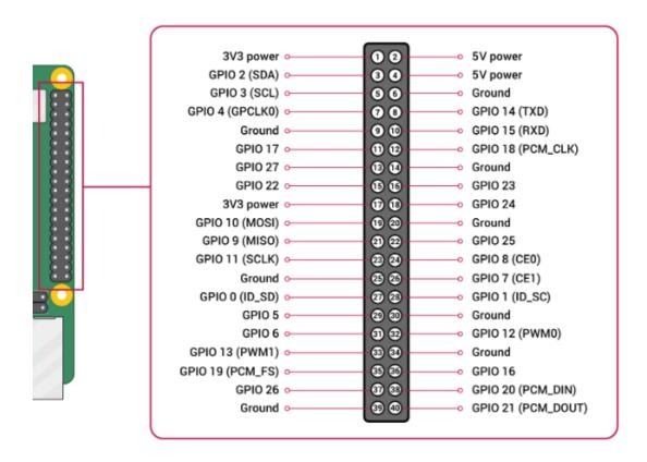
The 40-PIN header on ED-CM4NANO includes a debug serial port (GPIO14 = RX, GPIO15 = TX). Enable it via these steps.
