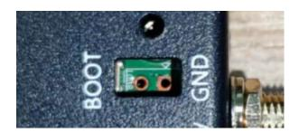
During the flashing process, short-circuit the BOOT and GND pins using jumper wires to enter flash mode. Remove the jumper wires immediately after flashing completes.
