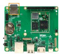
2. Press the Micro SD card gently into the slot until it ejects, then remove it.
