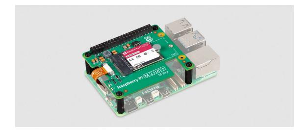
The Raspberry Pi SSD Kit bundles a Raspberry Pi M.2 HAT+ with a Raspberry Pi NVMe SSD. It unlocks outstanding performance for I/O intensive applications on Raspberry Pi 5, including super-fast startup when booting from SSD. The Raspberry Pi SSD Kit is available with 256GB or 512GB capacity, and includes a 16mm stacking header, spacers, and screws to enable fitting on Raspberry Pi 5 with the Raspberry Pi Active Cooler in place.
