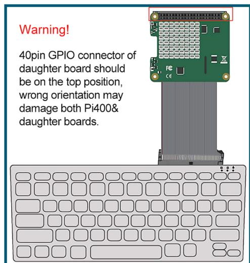
3. Please double check the orientation of daughter board and position of pin#1,2 & 40 base on the below picture before power on Pi 400.
