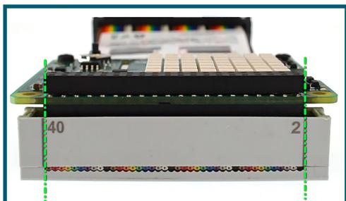
2. Align the pin# of daughter board with the mark on grey 40pin connector, make sure Pin#-1,2 & 40 on daughter is aligned with the mark-“1,2 & 40” on the grey male connector, insert the daughter board into grey connector.
