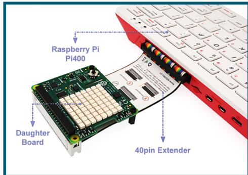
**Note:** The installation steps are identical for the Raspberry Pi 400, Pi 500, and Pi 500+, and are only illustrated here using the Pi 400 as an example.
